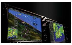
pletely new computer based, integrated system and it presents the flight instruments in a digital format rather than the customary steam gauges. Certainly, there is a level of similarity, the airplane flies the same as before but the presentation and volume of information is noticeably
